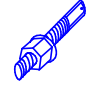
M12 Dynabolt provided for Frames 2438mm & taller to be fixed to the ground
