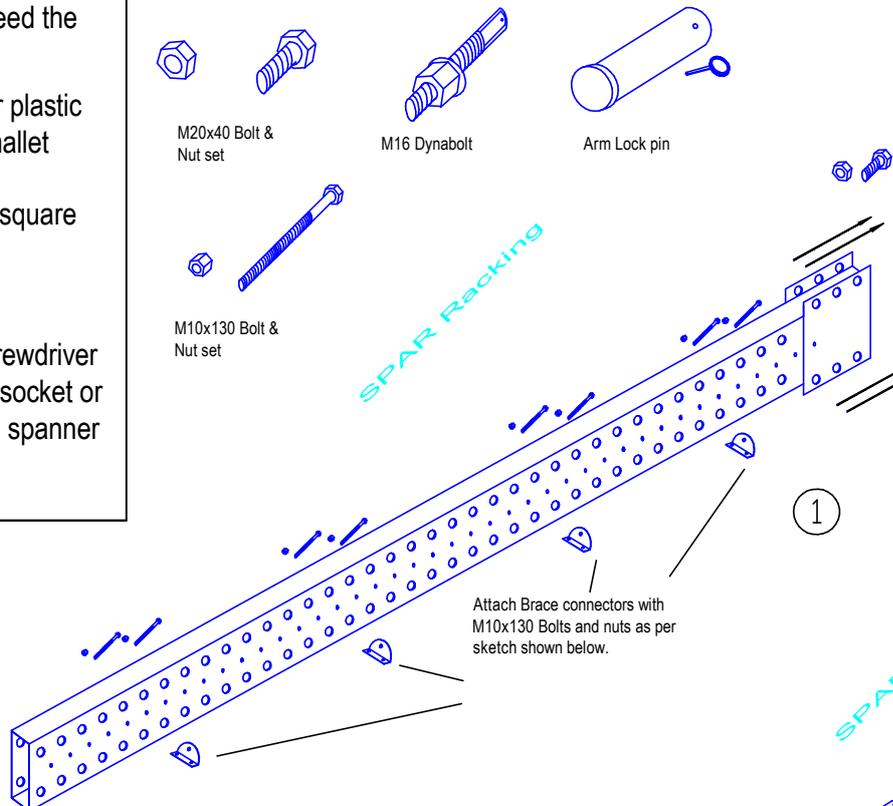
Attach Brace connectors with M10x130 Bolts and nuts as per sketch shown below.
