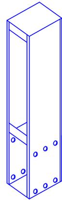
Slide column into base as shown and affix with 12 pcs M20x40 Bolt & Nut set.
